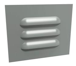
Hammond louver vent assembly,  $5.30 \times 6.30$ in (HxW), carbon steel, ANSI 61 gray, powder coat finish,  $2.88 \times 3.75$ in (HxW) cutout, for ventilation of metal enclosure. Aluminum filter mesh and mounting hardware included.
