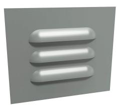
Hammond louver vent assembly,  $5.30 \times 6.30$  in (HxW), carbon steel, ANSI 61 gray, powder coat finish,  $2.88 \times 3.75$  in (HxW) cutout, for ventilation of metal enclosure. Aluminum filter mesh and mounting hardware included.
