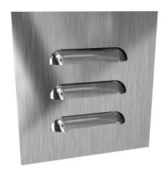
Hammond louver vent assembly,  $5.56 \times 5.30$ in (HxW), 304 stainless steel,  $3.00 \times 2.75$ in (HxW) cutout, for ventilation of metal enclosure. Aluminum filter mesh and mounting hardware included.
