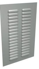
Hammond louver vent assembly,  $16.12 \times 10.30$  in (HxW), carbon steel, ANSI 61 gray, powder coat finish,  $13.25 \times 7.75$  in (HxW) cutout, for ventilation of metal enclosure. Aluminum filter mesh and mounting hardware included.
