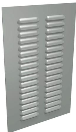
Hammond louver vent assembly, 16.12 x 10.30in (HxW), carbon steel, ANSI 61 gray, powder coat finish, 13.25 x 7.75in (HxW) cutout, for ventilation of metal enclosure. Aluminum filter mesh and mounting hardware included.
