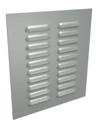
Hammond louver vent assembly,  $11.37 \times 10.30$ in (HxW), carbon steel, ANSI 61 gray, powder coat finish,  $8.50 \times 7.75$ in (HxW) cutout, for ventilation of metal enclosure. Aluminum filter mesh and mounting hardware included.
