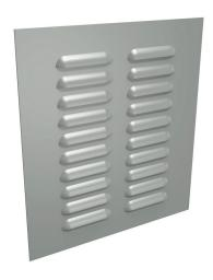
Hammond louver vent assembly,  $11.37 \times 10.30$ in (HxW), carbon steel, ANSI 61 gray, powder coat finish,  $8.50 \times 7.75$ in (HxW) cutout, for ventilation of metal enclosure. Aluminum filter mesh and mounting hardware included.
