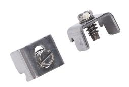
Hammond enclosure U-clamp assembly, replacement, 316 stainless steel. Package of 2. For use with 1418 and 1447 enclosures.
