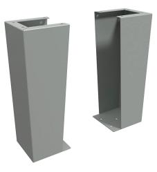
Hammond floor stand kit, 24in height, carbon steel, ANSI 61 gray, powder coat finish. For use with 8in deep enclosures. Includes (2) floor stands and mounting hardware.
