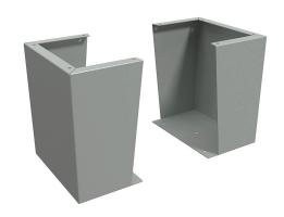
Hammond floor stand kit, 18in height, carbon steel, ANSI 61 gray, powder coat finish. For use with 16in deep enclosures. Includes (2) floor stands and mounting hardware.
