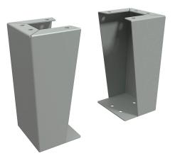
Hammond floor stand kit, 12in height, carbon steel, ANSI 61 gray, powder coat finish. For use with 6in deep enclosures. Includes (2) floor stands and mounting hardware.
