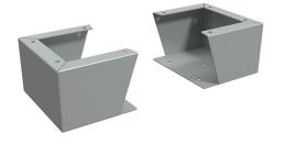
Hammond floor stand kit, 6in height, carbon steel, ANSI 61 gray, powder coat finish. For use with 10in deep enclosures. Includes (2) floor stands and mounting hardware.
