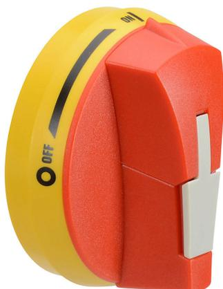
Socomec rotary handle, round, S00, red/yellow, external front or right side mount, 2-position, lockable in OFF only, defeatable, NEMA 4/4X.
