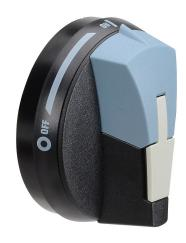
Socomec rotary handle, round, S00, black/blue, external front or right side mount, 2-position, lockable in OFF only, defeatable, NEMA 4/4X.
