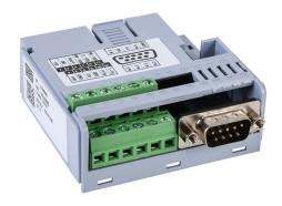
WEG Electric CFW500 series communication module, Modbus RTU and BACnet, 2 ports, (1) RS-232 (3-pin terminal) and (1) RS-485 (3-pin terminal) port(s). For use with WEG CFW500 series AC drives.
