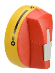
Socomec rotary handle, round, S00, red/yellow, external front or right side mount, 2-position, lockable in OFF only, defeatable, NEMA 1/3R/12.
