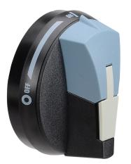
Socomec rotary handle, round, S00, black/blue, external front or right side mount, 2-position, lockable in OFF only, defeatable, NEMA 1/3R/12.
