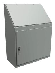
Hammond operator console, NEMA 12, 48 x 36 x 18in (HxWxD), freestanding, carbon steel, ANSI 61 gray, powder coat finish, single-door, 3-point keylocking handle.
