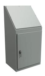
Hammond operator console, NEMA 12, 48 x 24 x 18in (HxWxD), freestanding, carbon steel, ANSI 61 gray, powder coat finish, single-door, 3-point keylocking handle.
