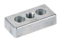
FATH transport/base plate, silver, 1 x 2in, 3/8-16 UNC, die-cast zinc, slot size 6. For use with 1 x 2in profile T-slotted rails. Mounting hardware included. Manufacturer part number: 093T25503/806RS01.
