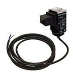
Eaton photoelectric sensor, rectangular, polarized retroreflective, visible red light emission, 45in sensing distance, selectable light-on/dark-on, solid state relay, potentiometer, 4-wire, pigtail.
