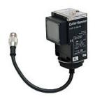
Eaton photoelectric sensor, rectangular, polarized retroreflective, visible red light emission, 16ft sensing distance, selectable light-on/dark-on, SPDT EM relay, potentiometer, 5-wire, 5-pin AC micro connector and 1/2in - 20UNF thread.
