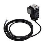
Eaton photoelectric sensor, rectangular, polarized retroreflective, visible red light emission, 16ft sensing distance, selectable light-on/dark-on, NPN/PNP, potentiometer, 4-wire, pigtail.
