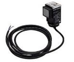
Eaton photoelectric sensor, rectangular, polarized retroreflective, visible red, 16ft sensing distance, selectable light-on/dark-on, solid state relay, potentiometer, 4-wire, pigtail.
