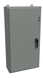
Hammond disconnect enclosure, NEMA 4/12/13, right flange, 48 x 25 x 10in (HxWxD), wall mount, carbon steel, ANSI 61 gray, powder coat finish, single-door, 3-point padlocking handle.
