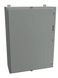
Hammond disconnect enclosure, NEMA 3R/4/12, right flange, 42 x 31 x 12in (HxWxD), wall mount, carbon steel, ANSI 61 gray, powder coat finish, single-door, stainless steel clamps.
