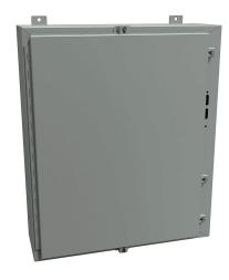
Hammond disconnect enclosure, NEMA 3R/4/12, right flange,  $30 \times 25 \times 8$  in (HxWxD), wall mount, carbon steel, ANSI 61 gray, powder coat finish, single-door, stainless steel clamps.
