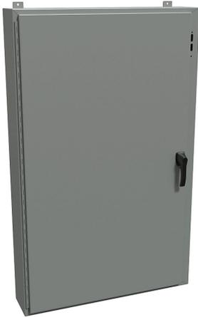
Hammond disconnect enclosure, NEMA 4/12/13, right flange, 60 x 37 x 8in (HxWxD), wall mount, carbon steel, ANSI 61 gray, powder coat finish, single-door, 3-point padlocking handle.
