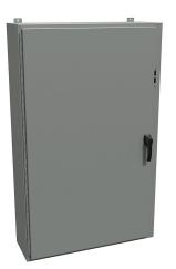
Hammond disconnect enclosure, NEMA 4/12/13, right flange, 60 x 37 x 12in (HxWxD), wall mount, carbon steel, ANSI 61 gray, powder coat finish, single-door, 3-point padlocking handle.
