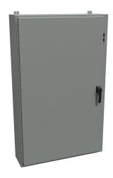
Hammond disconnect enclosure, NEMA 4/12/13, right flange, 60 x 37 x 10in (HxWxD), wall mount, carbon steel, ANSI 61 gray, powder coat finish, single-door, 3-point padlocking handle.
