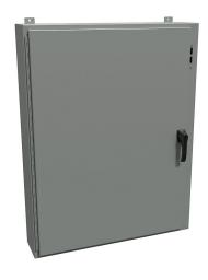
Hammond disconnect enclosure, NEMA 4/12/13, right flange, 48 x 37 x 8in (HxWxD), wall mount, carbon steel, ANSI 61 gray, powder coat finish, single-door, 3-point padlocking handle.
