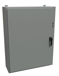
Hammond disconnect enclosure, NEMA 4/12/13, right flange, 48 x 37 x 12in (HxWxD), wall mount, carbon steel, ANSI 61 gray, powder coat finish, single-door, 3-point padlocking handle.
