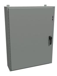
Hammond disconnect enclosure, NEMA 4/12/13, right flange, 48 x 37 x 10in (HxWxD), wall mount, carbon steel, ANSI 61 gray, powder coat finish, single-door, 3-point padlocking handle.
