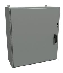
Hammond disconnect enclosure, NEMA 4/12/13, right flange, 42 x 37 x 16in (HxWxD), wall mount, carbon steel, ANSI 61 gray, powder coat finish, single-door, 3-point padlocking handle.
