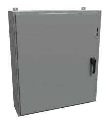
Hammond disconnect enclosure, NEMA 4/12/13, right flange, 42 x 37 x 10in (HxWxD), wall mount, carbon steel, ANSI 61 gray, powder coat finish, single-door, 3-point padlocking handle.
