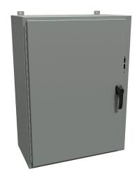
Hammond disconnect enclosure, NEMA 4/12/13, right flange, 42 x 31 x 16in (HxWxD), wall mount, carbon steel, ANSI 61 gray, powder coat finish, single-door, 3-point padlocking handle.
