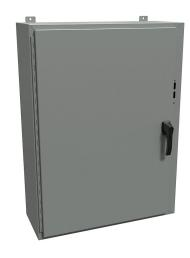
Hammond disconnect enclosure, NEMA 4/12/13, right flange, 42 x 31 x 12in (HxWxD), wall mount, carbon steel, ANSI 61 gray, powder coat finish, single-door, 3-point padlocking handle.
