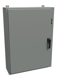
Hammond disconnect enclosure, NEMA 4/12/13, right flange, 42 x 31 x 10in (HxWxD), wall mount, carbon steel, ANSI 61 gray, powder coat finish, single-door, 3-point padlocking handle.
