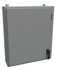
Hammond disconnect enclosure, NEMA 4/12/13, right flange,  $36 \times 31 \times 8in$  (HxWxD), wall mount, carbon steel, ANSI 61 gray, powder coat finish, single-door, 2-point padlocking handle.
