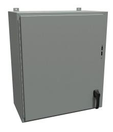
Hammond disconnect enclosure, NEMA 4/12/13, right flange, 36 x 31 x 16in (HxWxD), wall mount, carbon steel, ANSI 61 gray, powder coat finish, single-door, 2-point padlocking handle.
