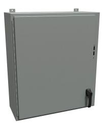
Hammond disconnect enclosure, NEMA 4/12/13, right flange,  $36 \times 31 \times 12$ in (HxWxD), wall mount, carbon steel, ANSI 61 gray, powder coat finish, single-door, 2-point padlocking handle.
