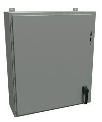
Hammond disconnect enclosure, NEMA 4/12/13, right flange, 36 x 31 x 10in (HxWxD), wall mount, carbon steel, ANSI 61 gray, powder coat finish, single-door, 2-point padlocking handle.
