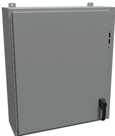
Hammond disconnect enclosure, NEMA 4/12/13, right flange, 36 x 31 x 10in (HxWxD), wall mount, carbon steel, ANSI 61 gray, powder coat finish, single-door, 2-point padlocking handle.
