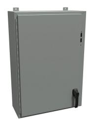
Hammond disconnect enclosure, NEMA 4/12/13, right flange, 36 x 25 x 10in (HxWxD), wall mount, carbon steel, ANSI 61 gray, powder coat finish, single-door, 2-point padlocking handle.
