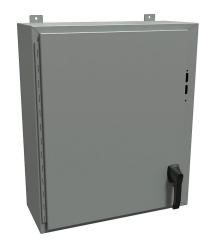
Hammond disconnect enclosure, NEMA 4/12/13, right flange,  $30 \times 25 \times 10$  in (HxWxD), wall mount, carbon steel, ANSI 61 gray, powder coat finish, single-door, 2-point padlocking handle.
