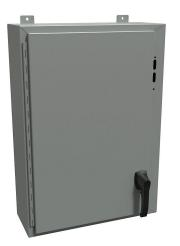
Hammond disconnect enclosure, NEMA 4/12/13, right flange,  $30 \times 21 \times 8in$  (HxWxD), wall mount, carbon steel, ANSI 61 gray, powder coat finish, single-door, 2-point padlocking handle.
