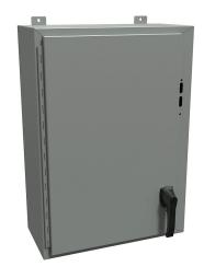
Hammond disconnect enclosure, NEMA 4/12/13, right flange,  $30 \times 21 \times 10$  in (HxWxD), wall mount, carbon steel, ANSI 61 gray, powder coat finish, single-door, 2-point padlocking handle.
