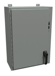
Hammond disconnect enclosure, NEMA 4/12/13, right flange, 30 x 21 x 10in (HxWxD), wall mount, carbon steel, ANSI 61 gray, powder coat finish, single-door, 2-point padlocking handle.
