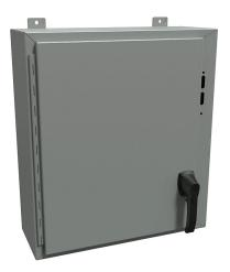
Hammond disconnect enclosure, NEMA 4/12/13, right flange,  $24 \times 21 \times 8in$  (HxWxD), wall mount, carbon steel, ANSI 61 gray, powder coat finish, single-door, 2-point padlocking handle.
