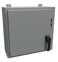
Hammond disconnect enclosure, NEMA 4/12/13, right flange, 20 x 21 x 8in (HxWxD), wall mount, carbon steel, ANSI 61 gray, powder coat finish, single-door, 2-point padlocking handle.
