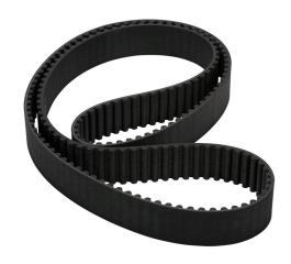
SureMotion timing belt, 8mm 8M pitch, 30mm wide, 180 tooth, 1440mm pitch length (circumference), neoprene, fiberglass reinforced.
