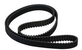
SureMotion timing belt, 8mm 8M pitch, 20mm wide, 180 tooth, 1440mm pitch length (circumference), neoprene, fiberglass reinforced.
