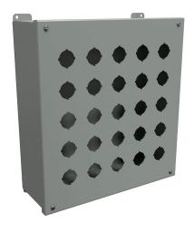
Hammond pushbutton enclosure, 25 holes, 30mm, NEMA 12/13,  $14 \times 13 \times 5$  in (HxWxD), wall mount, carbon steel, ANSI 61 gray, powder coat finish, hinged screw cover.
