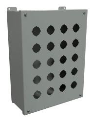
Hammond pushbutton enclosure, 20 holes, 30mm, NEMA 12/13, 14 x 11 x 5in (HxWxD), wall mount, carbon steel, ANSI 61 gray, powder coat finish, hinged screw cover.
