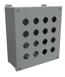
Hammond pushbutton enclosure, 16 holes, 30mm, NEMA 12/13, 12 x 11 x 5in (HxWxD), wall mount, carbon steel, ANSI 61 gray, powder coat finish, hinged screw cover.
